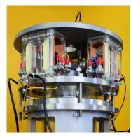
routinely test both 70mm and 100mm diameter specimens. Each cell is capable of being equipped with three pairs of bender elements to determine shearwave velocities in up to three directions,
