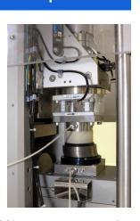
Our **Direct Simple Shear (DSS)** apparatus can perform both **static** and **cyclic** tests with sinusoidal or custom loading profile. Tests can be carried out controlling either the **shear load** or the **shear strain**. Platens are available with **pins** or **ridges** to best prevent slippage
