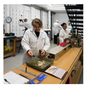
Our team can perform index testing (such as Torvane and pocket penetrometer) for rapid assessment of shear strength and unconfined compression strength of cohesive soils. We can also undertake undisturbed and disturbed sub-sample preparation for other laboratory testing requirements (such as Triaxial, Oedometer, Laboratory Vane, Shearbox, Particle Size Distribution and Atterberg limits etc).
