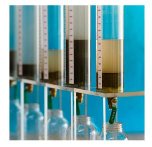
**Undrained Settling** measures how the fines settle out of a homogenous slurry that has been either supplied by the client, or mixed by Geolabs to a specified pulp density from dried materials. Where permitted by the materials, two properties are measured over time during the test: the gradually rising height of the settled materials, and the gradually lowering height of the fines above which there is clear water.
