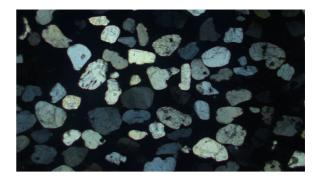
In concrete aggregates, petrographic examinations are used to characterize the rock type, name, and its suitability for use as a concrete aggregate. This helps to identify the constituents that are susceptible to alkali silica reactions in concrete and also when used in freeze/thaw environments.
