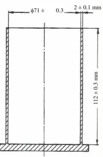
Figure 1 a) Mould and funnel recommended, b) Dimensions of the mould.
