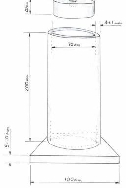
volume and cross-sectional area of the mould shall be calibrated before initial use. Calibration of the mould shall be carried out annually or after 250 tests (equivalent to 500 runs) whichever occurs first. Determine the volume of the mould by both the direct-measurement method and by water filling method. If the difference between the volumes is greater than 0.5% the calibrations should be repeated. If after repeating the difference exceeds 0.5% then the mould should be replaced.
