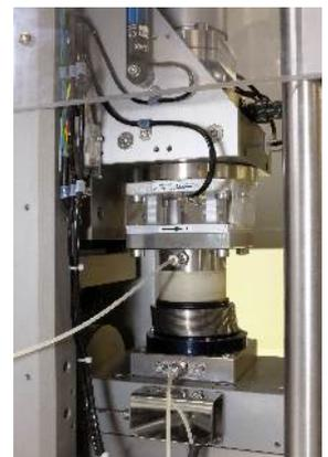
Our **Direct Simple Shear (DSS)** apparatus can perform both **static** and **cyclic** tests with sinusoidal or custom loading profile. Tests can be carried out controlling either the **shear load** or the **shear strain**. Platens are available with **pins** or **ridges** to best prevent slippage
